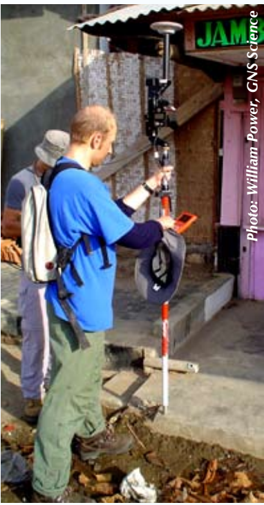
Dr Stefan Reese of NIWA using the ground-based differential RTK-GPS to take detailed topographical measurements of tsunami damage in Java.
